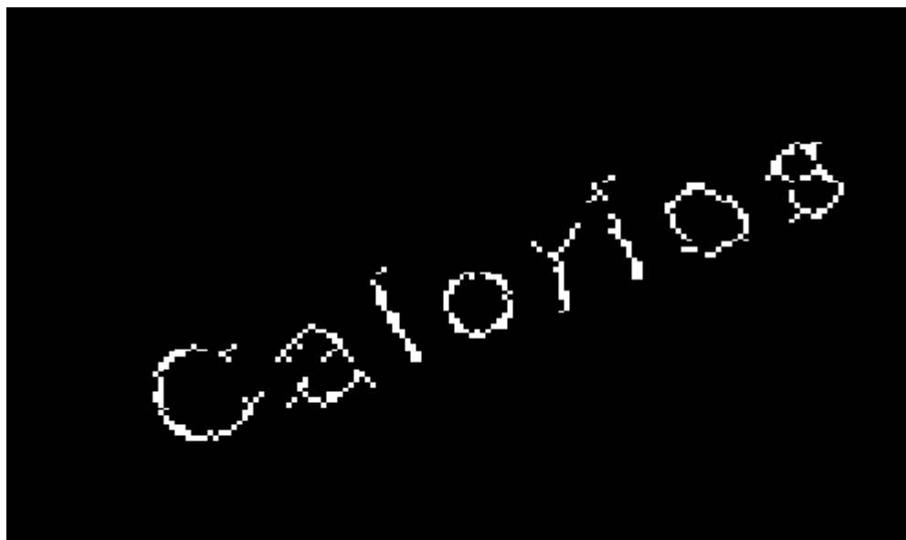
Figure 5.6 A cropped word from a text row produced after line segmentation step
